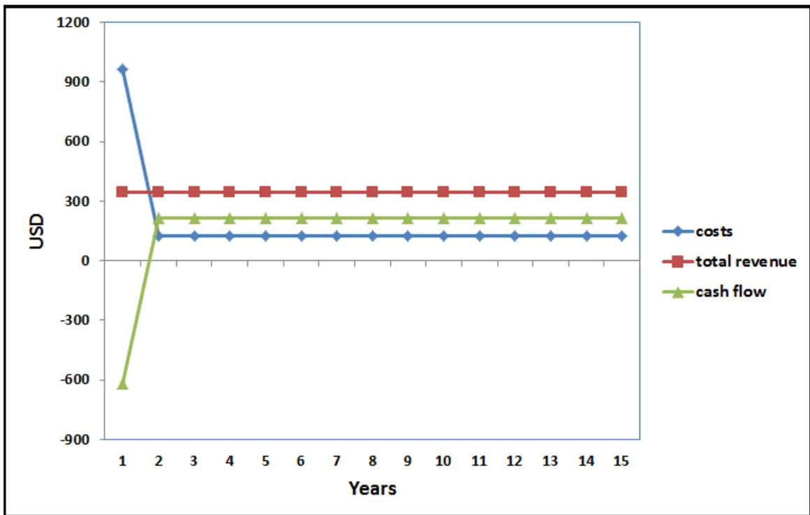
Figure (3) Total costs, revenues and cash flows of a biogas unit that uses animal waste without discounting factors
