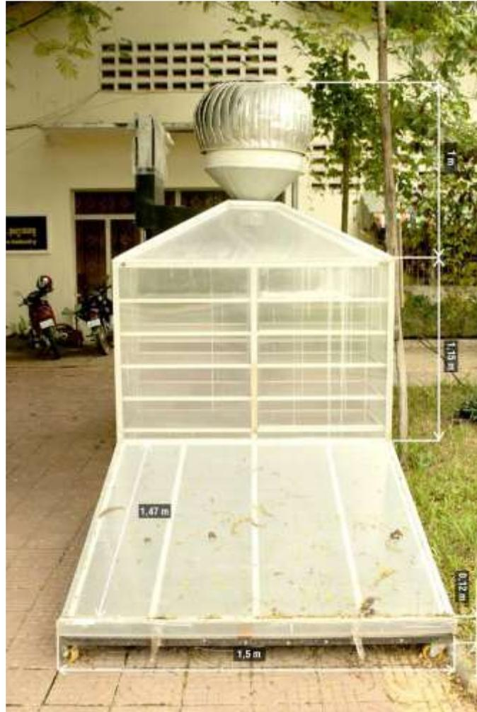
**Figure 3.5 Photograph of a natural convection solar dryer**
