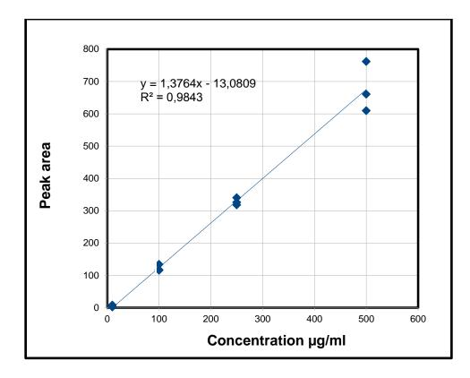
Figure 10 Calibration curve for resveratrol quantification
