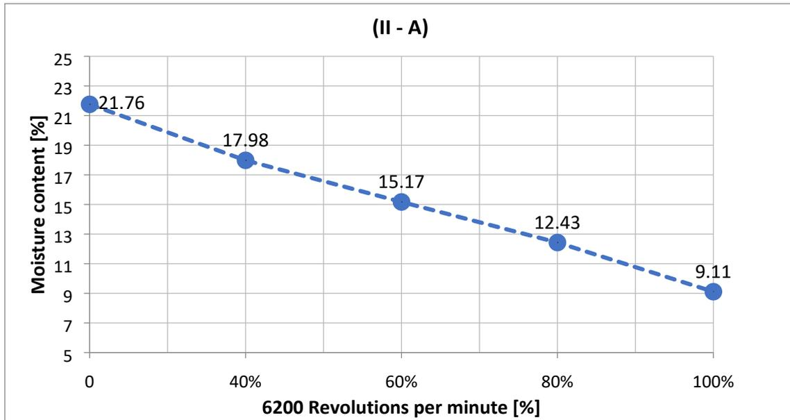
**Figure 33.** Moisture content related to rotors speed for (II – A)
