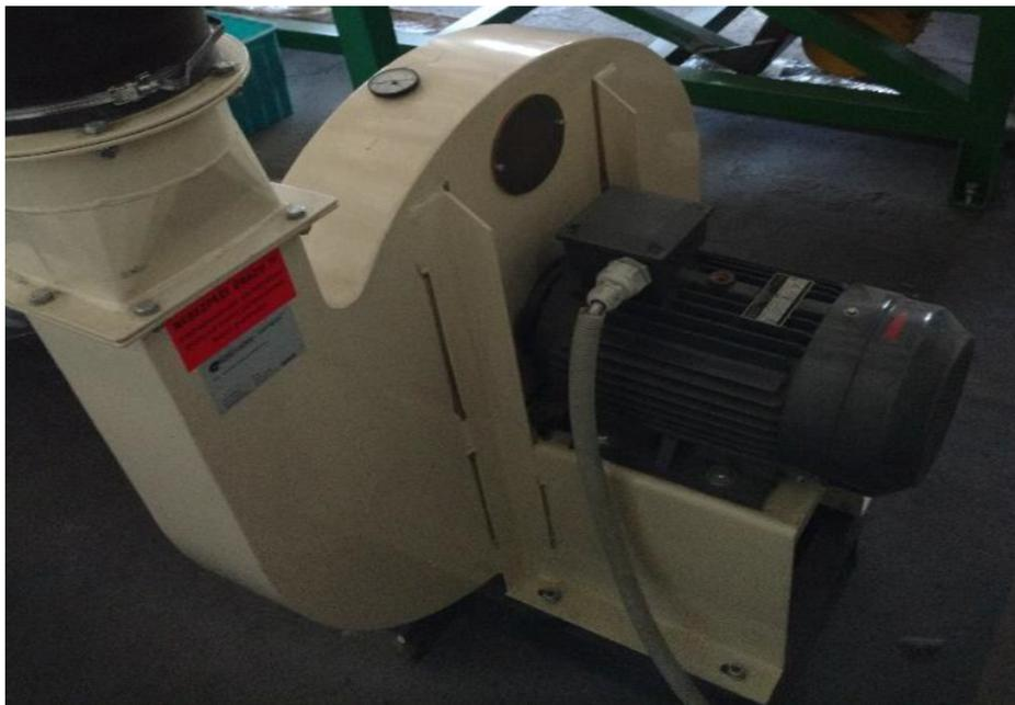
**Figure 17.** CIPRES transport ventilator
