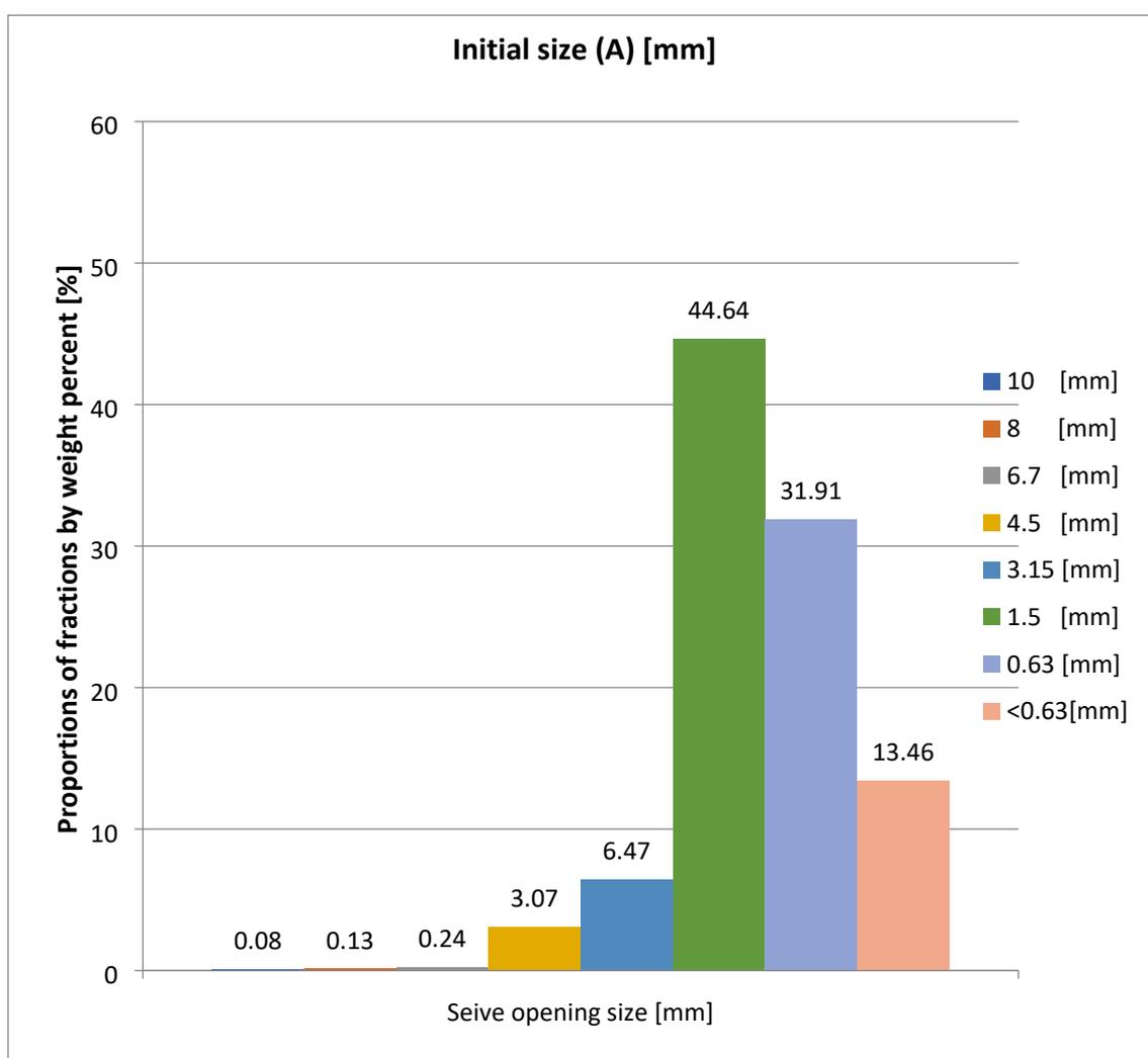
**Figure 8.** Initial particle size distribution for Apple tree wood
