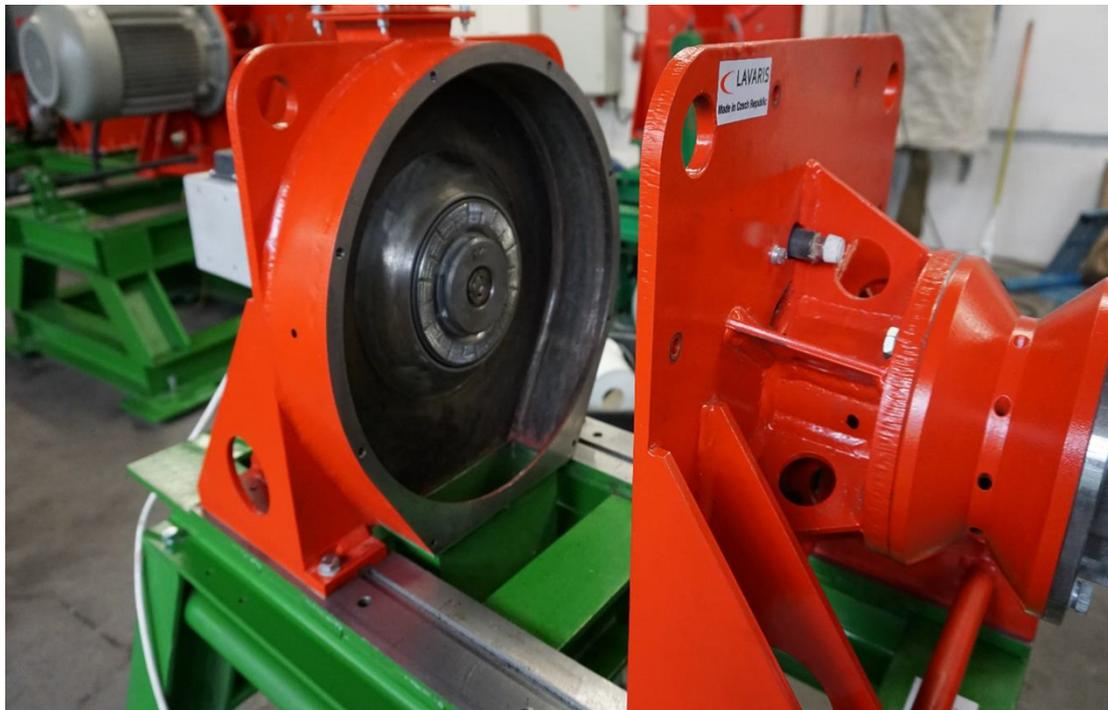
**Figure 6.** High speed counter-direction mill LAV 150/2R
