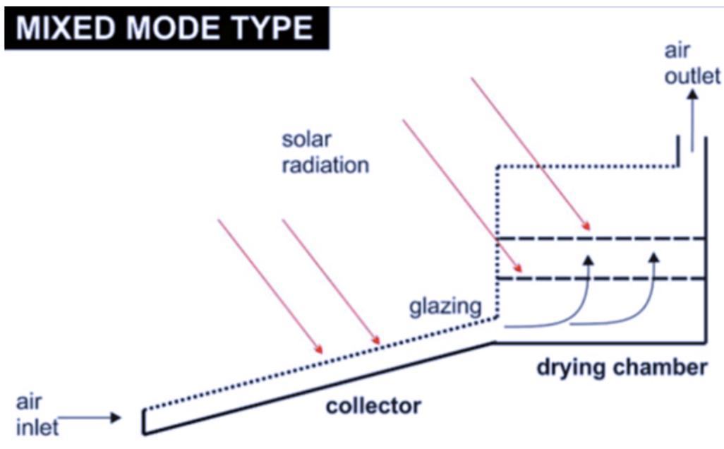
Figure 5. Mixed mode dryer. Source: Prakash et al. (2017)
