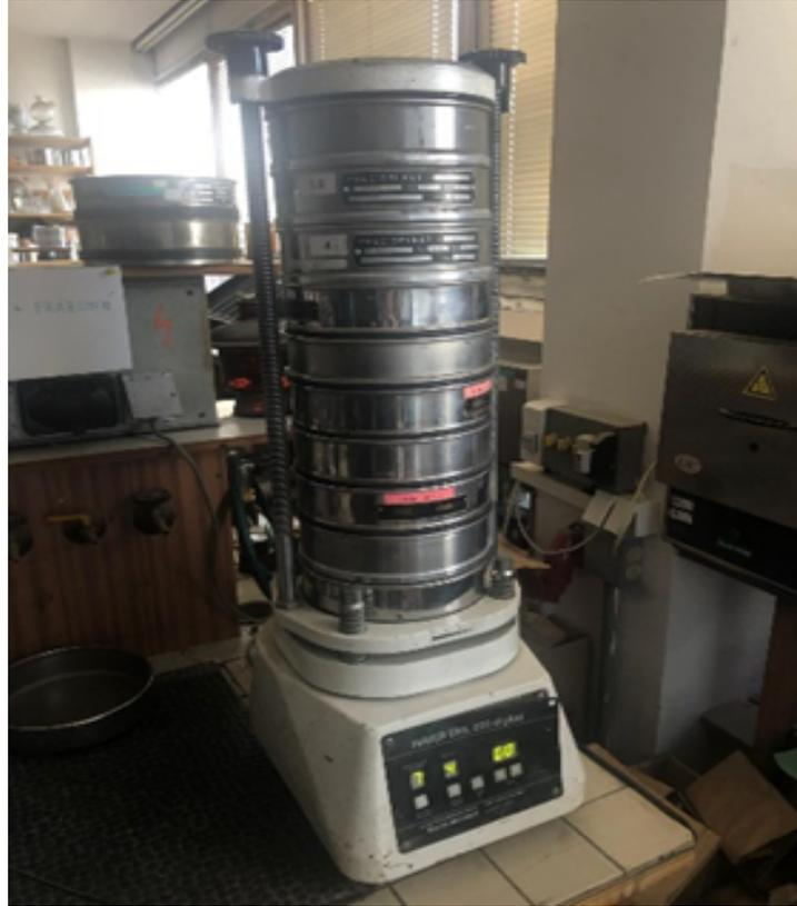
**Figure 22.** Laboratory sieve shaker HAVER EML 200
