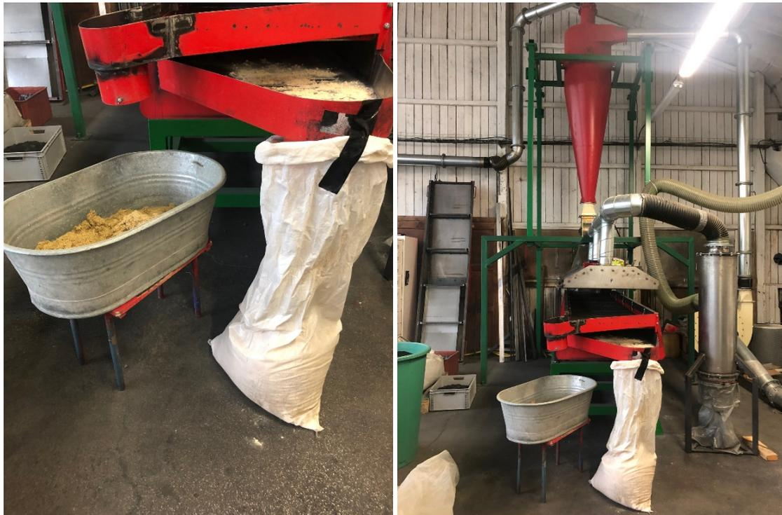
Figure 19. Vibrating screener
