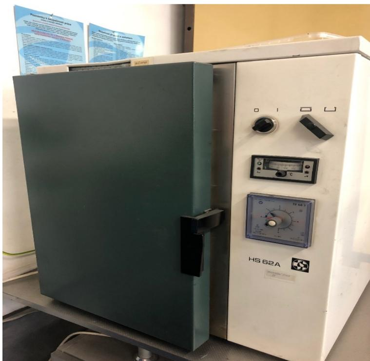
**Figure 24.** Laboratory dryer HS 62A
