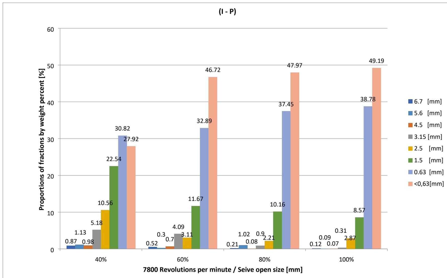
**Figure 44.** Particle size distribution according to rotor speed for (I – P) [mm]
