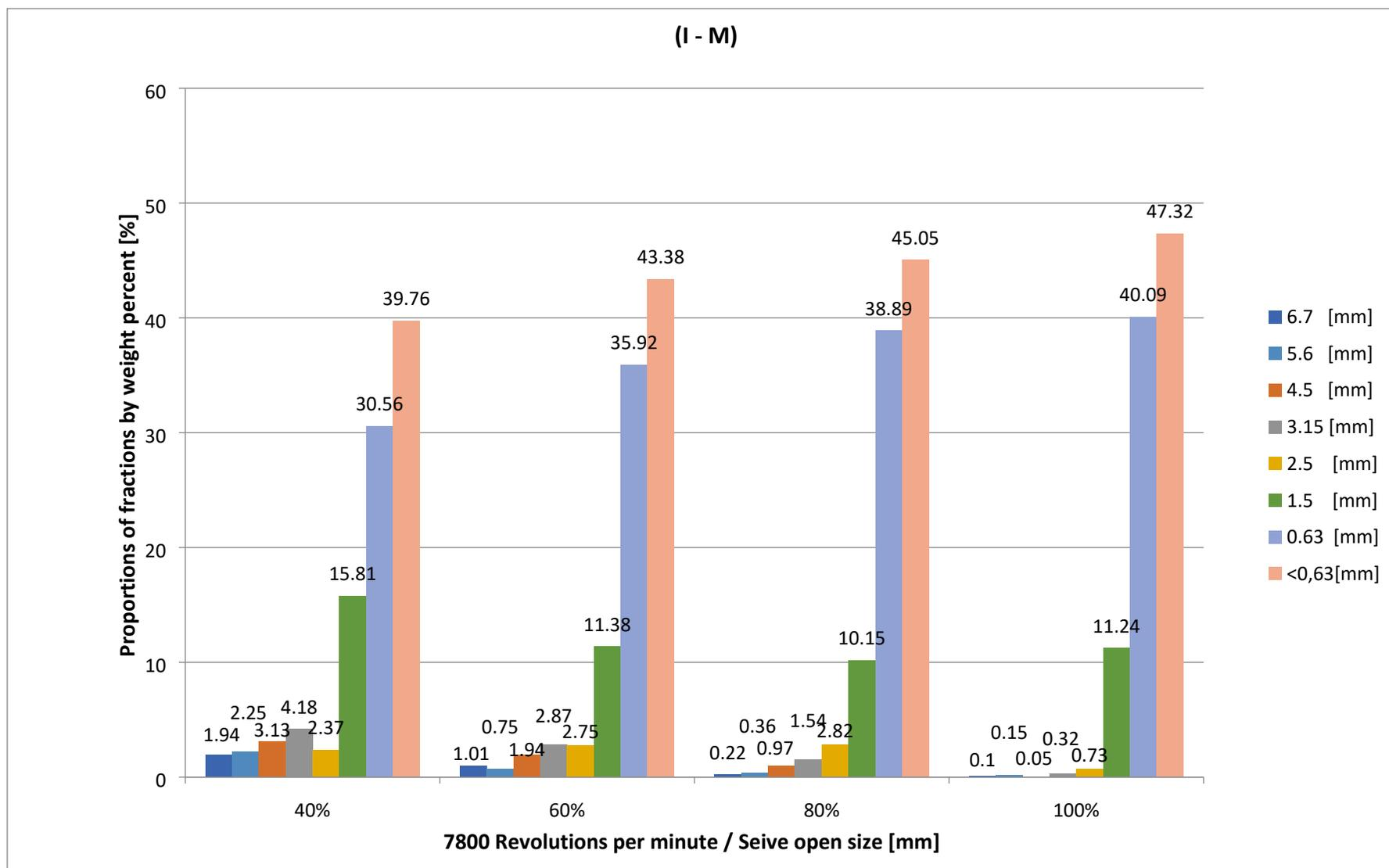
**Figure 36.** Particle size distribution according to rotor speed for (I – M) [mm]
