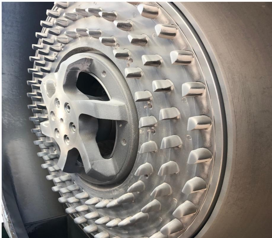
**Figure 7.** Pin-type rotor of HSM LAV 650/2R
