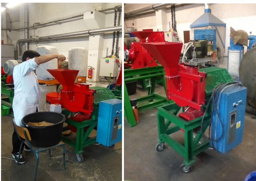
**Figure 13.** High-speed multilevel single rotor mill LAV 400/1R
